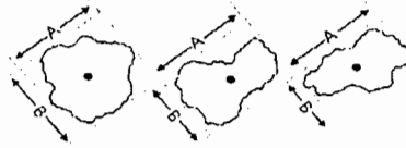
Fig. 1 Add A and B together and divide by 2 to get the Spread.
